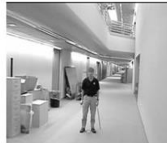
Figure 1(b). A Closed-Circuit Television Image Not Likely to be Suitable for Personal Identification.
